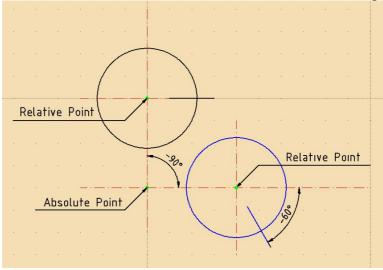
The original entity is in black, the result of the double rotation is blue. The angles used are respectively -90° and -60°. The reference points are named.
