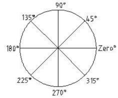
The example above shows 8 lines drawn with "Snap Center", length equal to radius and the angles as indicated.
